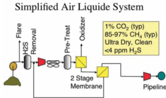
Figure 1. A process flow diagram for a simplified Air Liquide system
