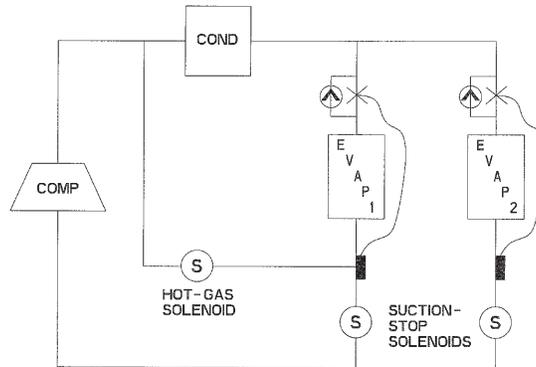
**Note:** When used in suction applications, a valve with a low pressure drop should be used (less than two pounds-per-square-inch differential [psid]). Piston-type pilot valves often have a minOPD that exceeds this. For this reason, diaphragm valves are recommended for suction service.
