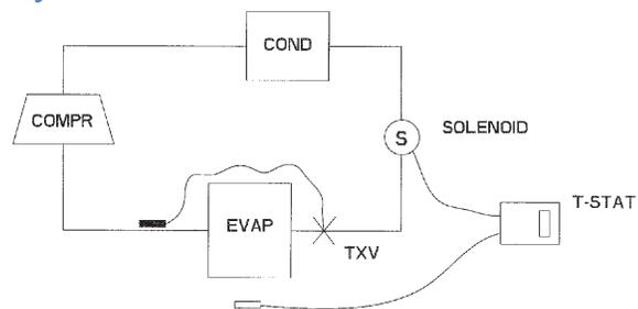
**Note:** This type of cycle is ideal in systems with large charges, because it prevents the possibility of the compressor starting with a large amount of liquid in the evaporator.
