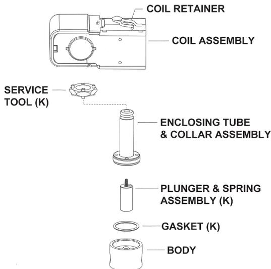
"K" indicates the part is supplied in the valve repair kit.
